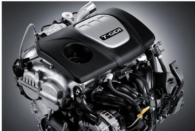
Another problem of T-GDI motors can be LSPI. See also the MPM OEM Newsletter number 04-2019. LSPI stands for "low speed pre-ignition", (at low rpm and high load, the fuel mixture ignites too early), which can cause enormous engine damage (such as piston damage). By using other additives in the lubricating oil, LSPI can be prevented. LSPI tests are therefore included in the latest (OEM) specifications.
